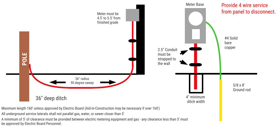
All single meter bases with separate disconnect unit must be grounded at meter base.
