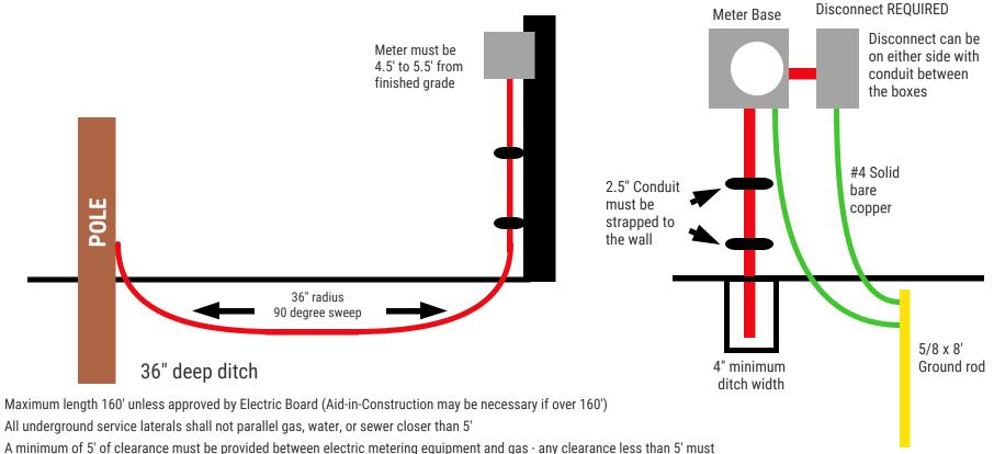
All underground service laterals shall not parallel gas, water, or sewer closer than 5'
